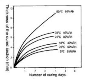
Relationship between curing speed and temperature/humidity
