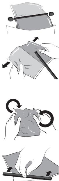
1. A pre-weighed pack containing the correct amount of each component, separated by a clip.
