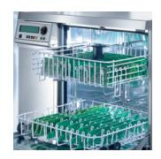
Cleaning processes can be referred to as batch or in-line processes. Batch systems refer to a batch of PCBs taken through the entire process, whether it is ultrasonic or dishwasher application, for example. Cleaning processes can also be set up as in-line systems where PCBs are constantly transferred through each stage and a continuous production line is formed.
