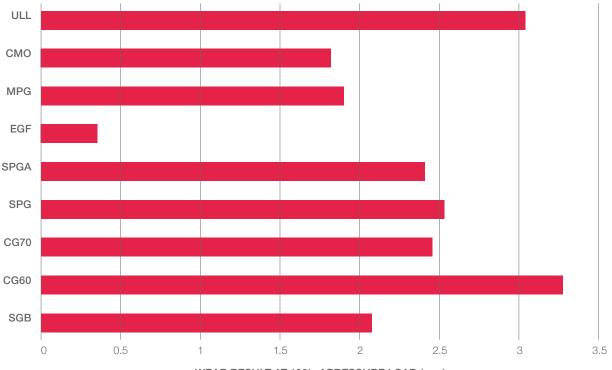
WEAR RESULT AT 100kgf PRESSURE LOAD (mm)
