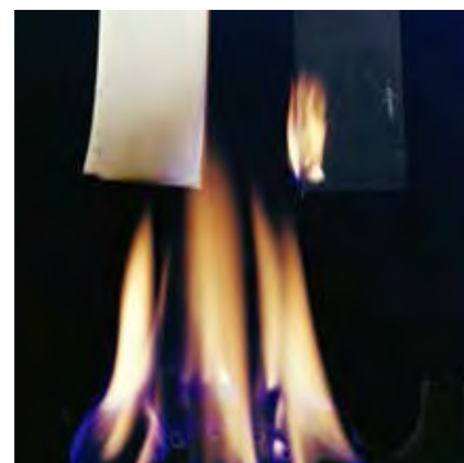
Flame resistance testing left: silicone rubber / right: organic rubber
