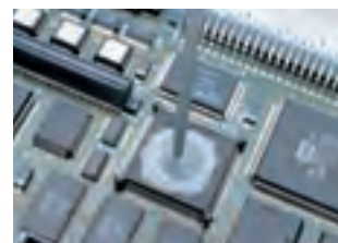
Thermal interface for CPUs
