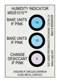
"Humidity Indicator Card (HIC) A card on which a moisture-sensitive chemical is applied such that it will make a significant, perceptible change relative humidity in color (hue), typically from blue (dry) to pink (wet) when the indicated relative humidity is exceeded. Note: The HIC is packed inside the moisture-barrier bag, along with a desiccant, to aid in determining the level of moisture to which the moisture-sensitive devices have been subjected." [J-STD- 033C section 1.5.7]
