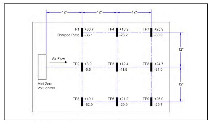
Figure 5. Neutralization (Discharge) Times
