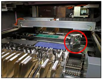
Figure 4. Using the Mini Zero Volt Ionizer inside automated machinery.
