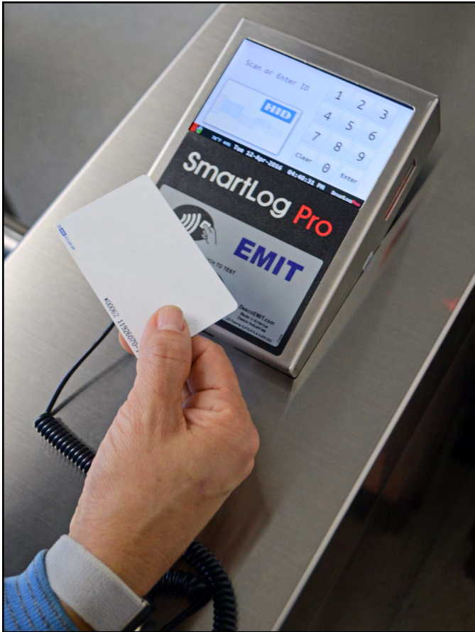
Figure 4. Holding a proximity badge in front of the RFID icon on the SmartLog Pro®
