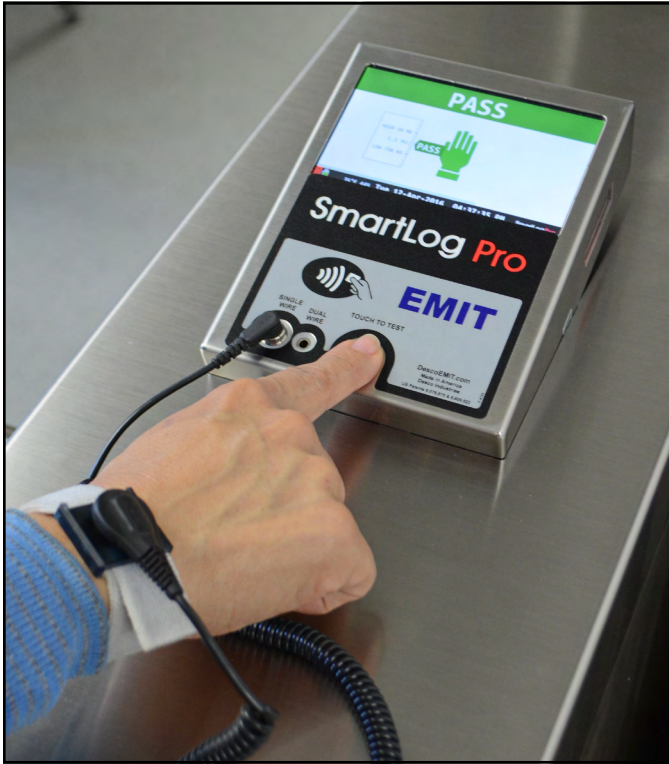
Figure 6. Performing a single-wire wrist strap test
