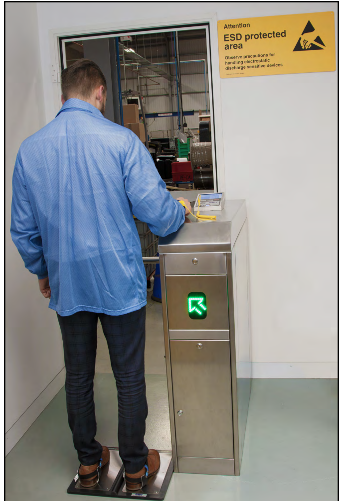
Figure 5. Performing a footwear and wrist strap test
