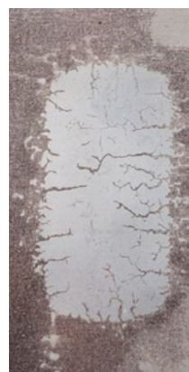
Photographs illustrating the difference in performance following thermal shock testing between -40°C and +125°C.
